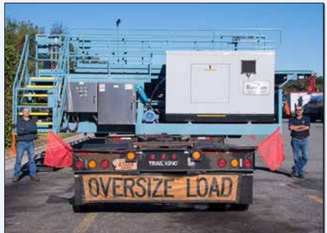
The 94,000-pound scissor-lift platform stretched 110-feet long and spanned 24 feet 6 inches – taking up two lanes of highway.
